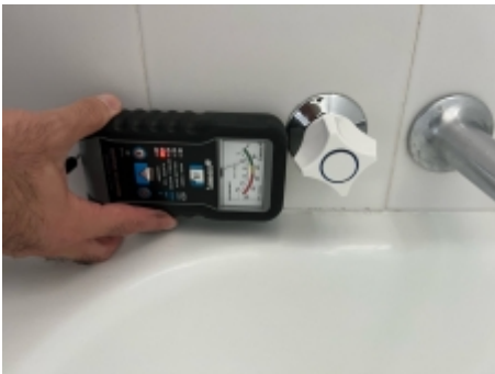
Showing examples of moisture meter readings taken on site, where the level recorded did not show an elevated reading.
